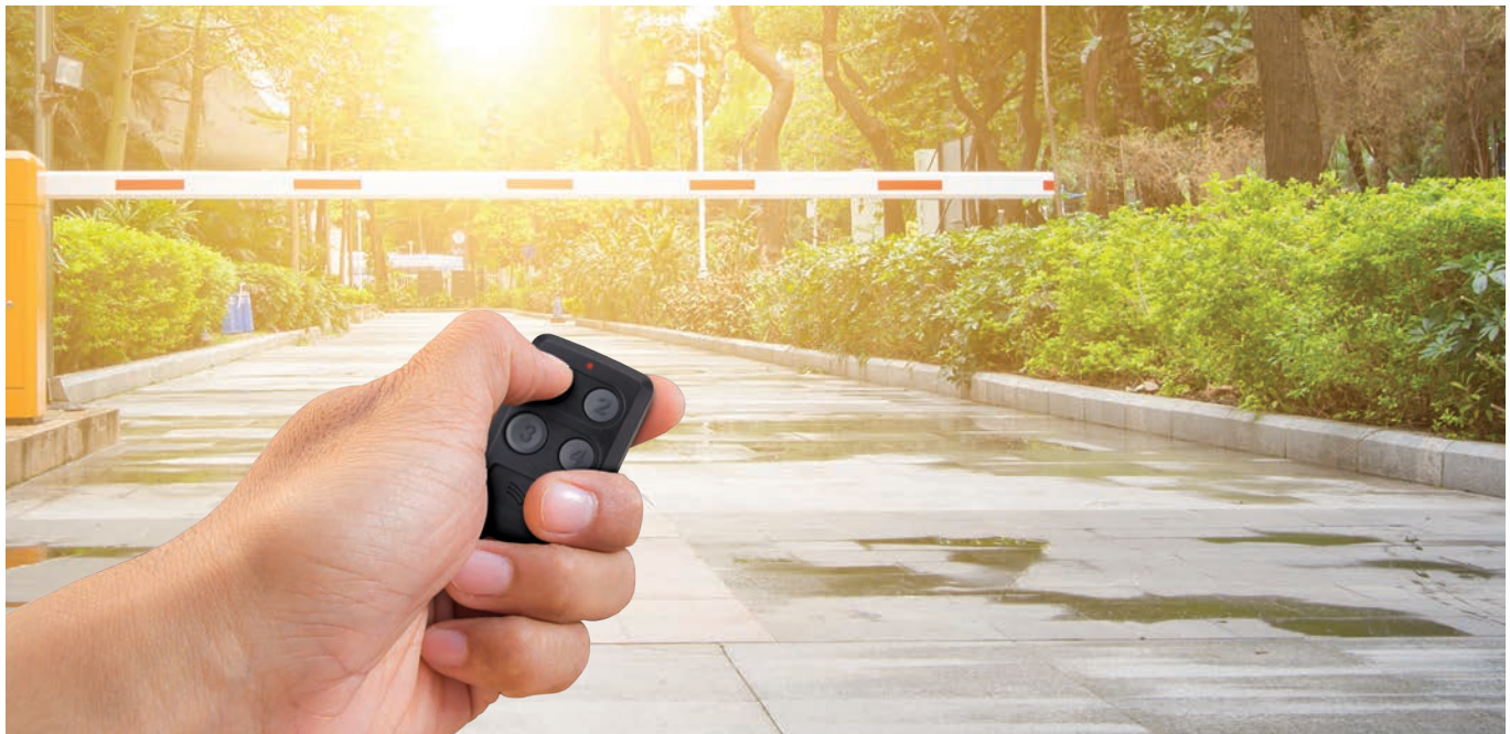
Long-range transmitters with a range of up to 200 feet allow a receiver to be placed in a secure location—out of sight and out of harm's way.
