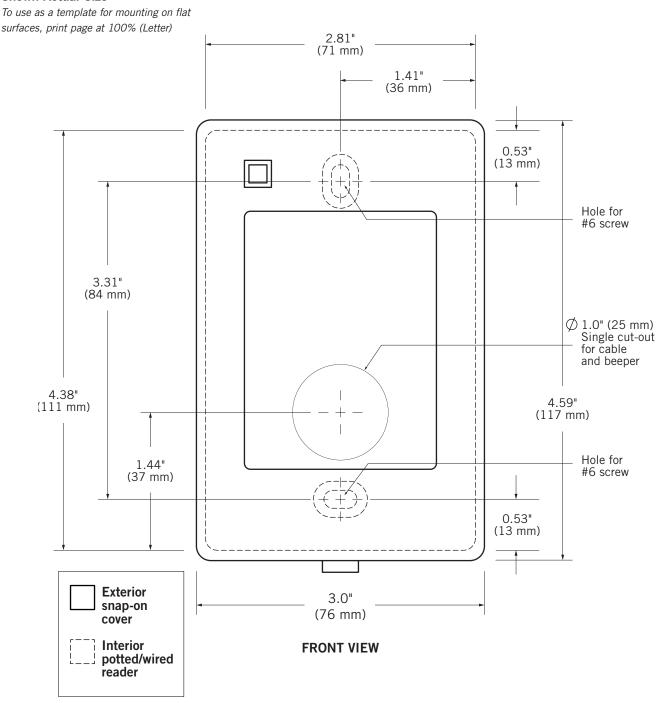
Be sure to use appropriate tools and proper safety equipment during installation. Farpointe Data reserves the right to change specifications without notice.
