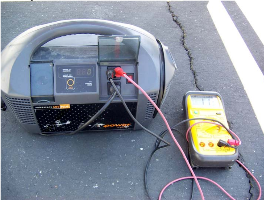
Close up of DC-AC Inverter
